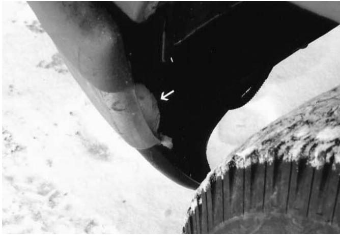
Figure 1. Digital image of a PRRSV-positive carrier attached to the left front wheel well of the study vehicle. The carrier is denoted by the arrow.
